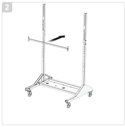
Install the upper cross brace between the inside frame rails with the four each M8 x 60mm button head Allen screws and flat washers supplied. Tighten all eight M8 x 60mm button head Allen screws to create a firm frame structure at this time.
