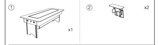
1 To install Axessline Quickbox, a cut out hole must be in place at the desired position of the table. Continue by vertically placing the box (1) inside the hole as illustrated below.
