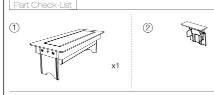
● To install Axessline Quickbox, a cut out hole must be in place at the desired position of the table. Continue by vertically placing the box① inside the hole as illustrated below.
